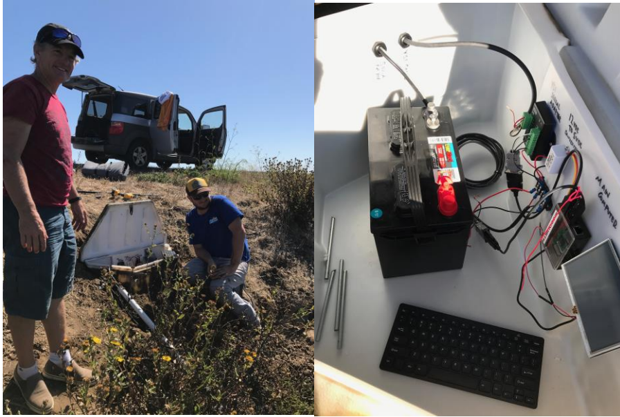
Figure 1a and 1b. (1a) John Haskins (ESNERR) and Jason Adelaars (MLML) are working on the MCSQUIRTS system at Highway 1. (1b) The box contains batteries and computer system that store data and power the YSI EXO sonde, SUNA nitrate sensors, and ADCP.
